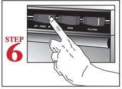
Turn Power Switch to "ON" position. Hold down "FILL" Switch until water reaches spray arm level.
