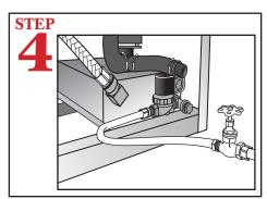
Connect dishmachine to hot water source, recommended 140° (120° minimum temperature required) using a 1/2" connector.
