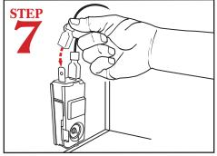
Reconnect thermostat wire. Set temperature at 120°F - 140°F.
