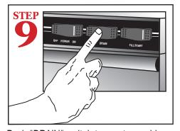
Push "DRAIN" switch to empty machine.
