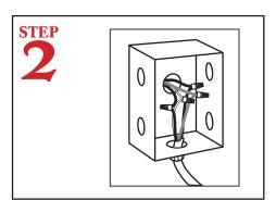
To connect hard wire power supply from the dishmachine to the power box, remove front panel.
