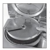
Next, fit the corresponding slicing disc (straightedged blade) and rotate in a clockwise direction to ensure that it is correctly positioned.
