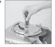
Position the automatic hopper on the motor base. The fastening hook is now facing you on your right.
