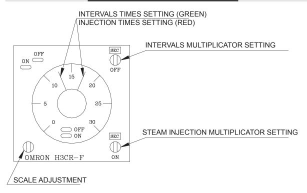
By pushing the GREEN button, the button will light up and the automatic system injection will start. The injection will be done as per the pre-adjustment time on the automatic steam timer. The standard steam timer (white light) will light up during the steam injection. Push the RED button to stop the automatic steam injection and then, the GREEN button will turn off.
